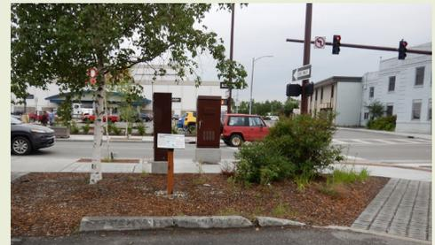
Transit Park is using green infrastructure such as stormwater trees and permeable pavers to help retain rainwater and soak it into the ground. Photo Credit: Alaska DOF.
