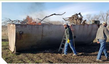
Loading trees and branches with a wheel loader into an oil tank biochar kiln. *Photo Credit: Kelpie Wilson*
