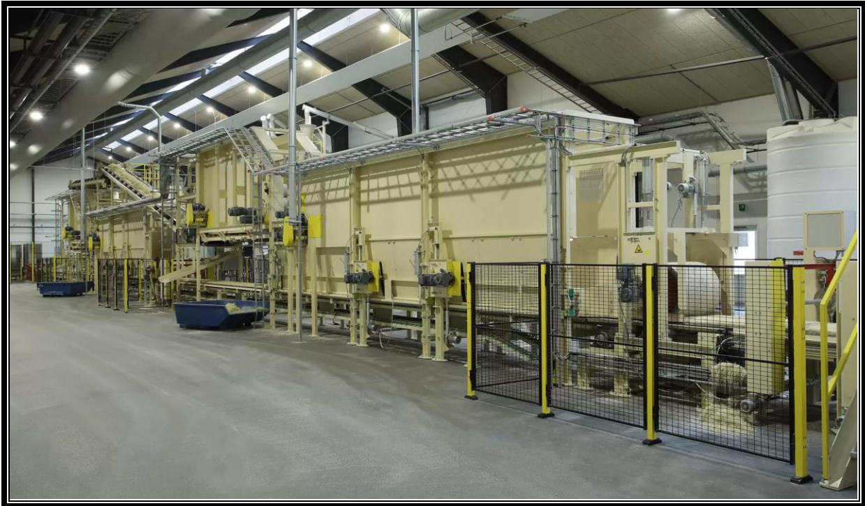
Figure 2.13 – The Main Forming Line Where the Wood Wool, Cement, and Accelerator Mixture is Formed into Panels
