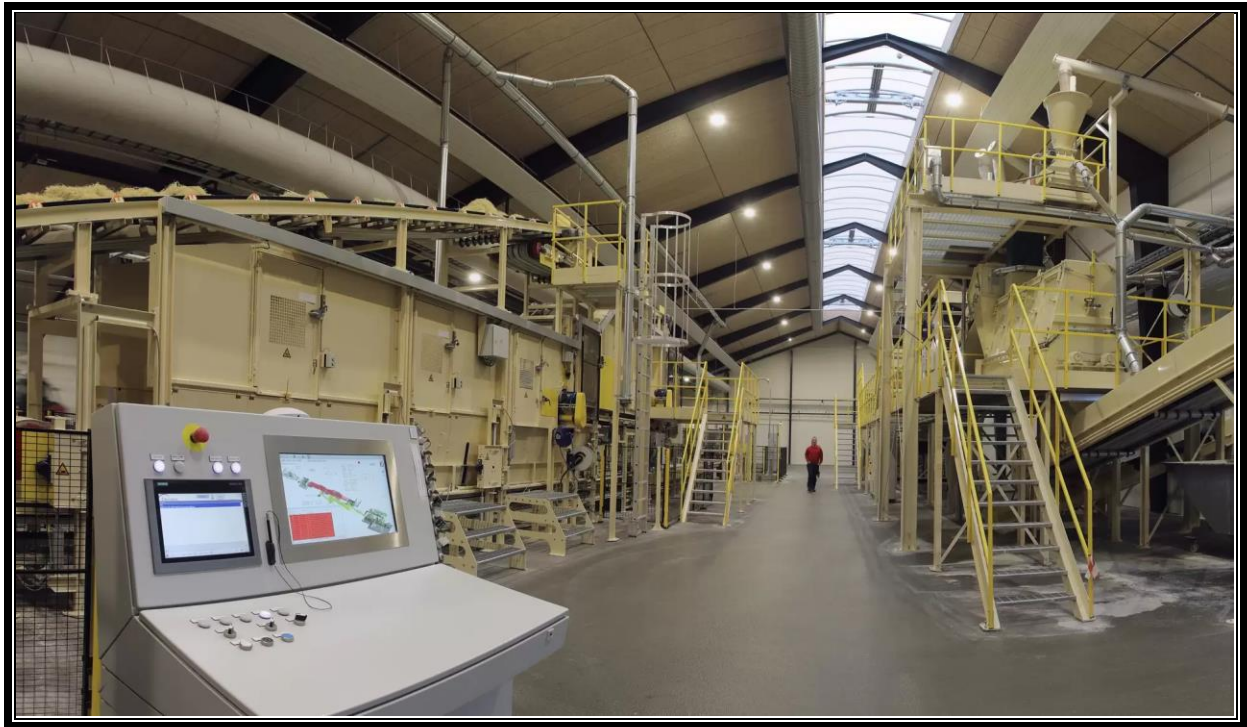
Figure 2.13 – The Main Forming Line Where the Wood Wool, Cement, and Accelerator Mixture is Formed into Panels
