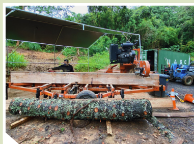
Plantation species being milled for the HWUT ADU at Kalani Hardwoods. Photo Credit: Hawai'i Wood Utilization Team
