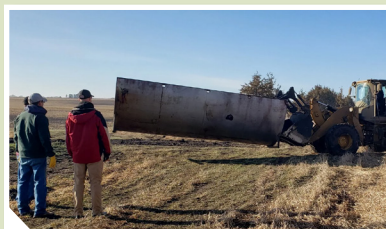
Moving half a surplus oilfield tank to be used as a flame-cap biochar kiln. Photo Credit: Kelpie Wilson
