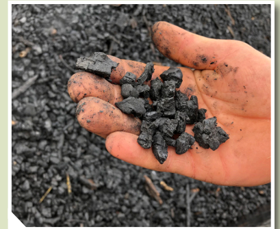
Char produced from waste tree material as part of the ROI Carbonator 500 Demonstration held near Haven, KS on Nov. 20, 2019. Photo Credit: Dave Bruton
