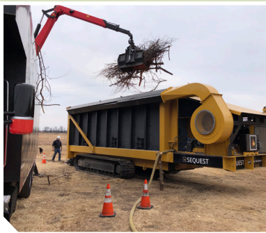
ROI Carbonator 500 being loaded with wood waste during the demonstration held near Haven, KS. Photo Credit: Dave Bruton
